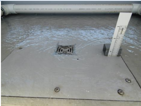
Weir Flow – 0.75 L/s (14 mm)
