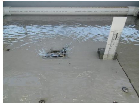
Orifice Flow – 1.5 L/s (50 mm)
