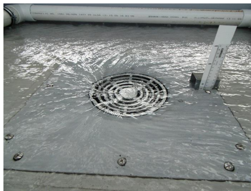
Weir Flow – 7 L/s (30mm)
