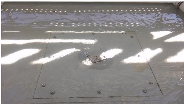
Weir flow - 1 L/s (50mm)
