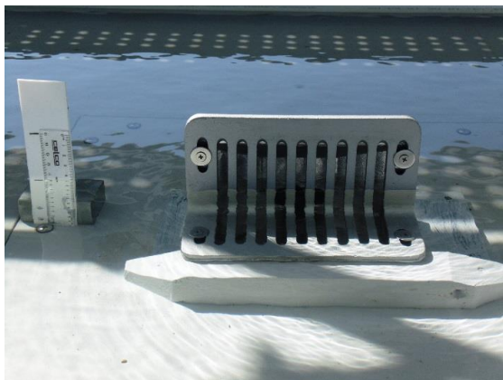
Weir Flow – 2 L/s (50mm)
