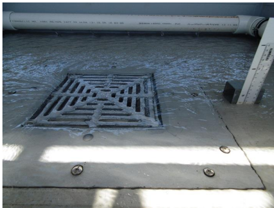
Weir Flow – 7 L/s (18mm)
