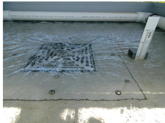
Surcharged Flow – 12 L/s (25mm)
