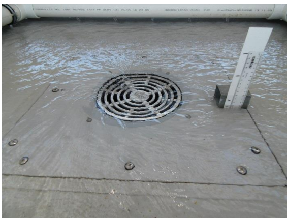
Weir Flow 6.0 L/s (35mm)
