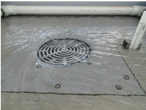
Weir Flow – 7 L/s (25mm)
