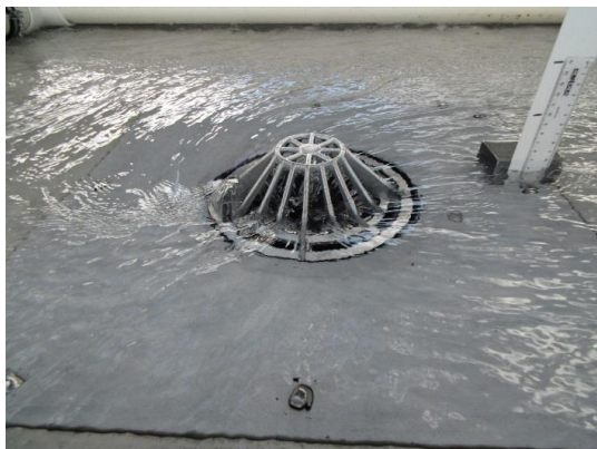
Weir Flow 8 L/s (37mm)
