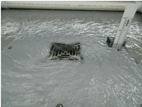
Weir flow - 2 L/s (35mm)
