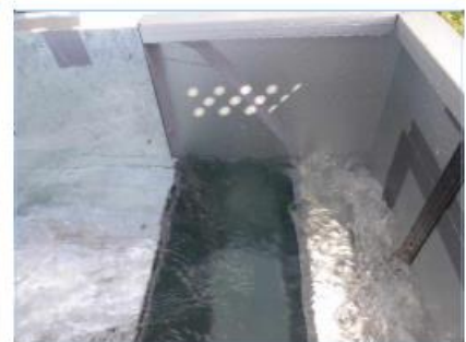
DB 400-1, Q = 16 l/s (box gutter slope - 1 in 200)
