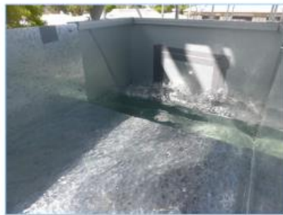
DB 500-1, Q = 16 l/s (box gutter slope - 1 in 200)
